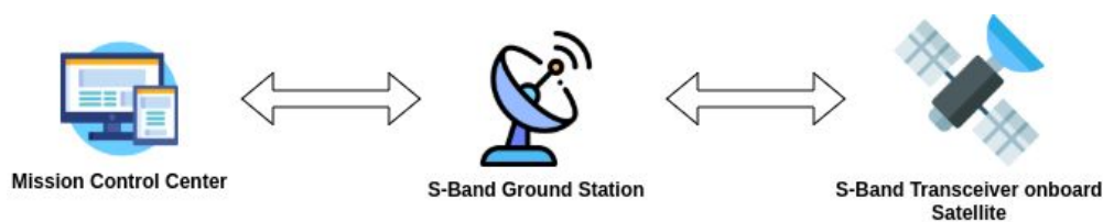
Figure 1: S-Band communications chain in upcoming CSUM's missions.
