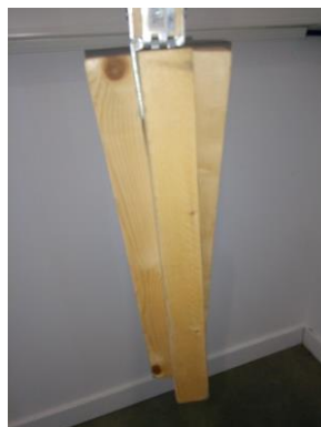
Figure 6-4 : Picture of the quadripod pole in transport configuration (before).
