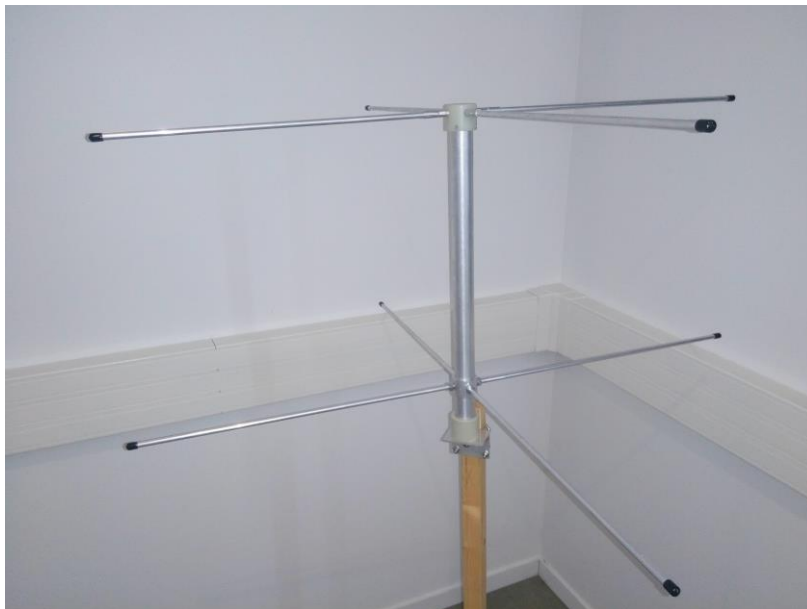
Figure 4-1 : Photo of the Turnstile antenna for VHF band.
