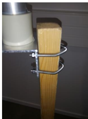
Figure 7-9 : Picture of the antenna fastening system around the quadripod pole.
