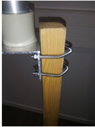
Figure 6-8 : Picture of the antenna fastening system around the quadripods pole
