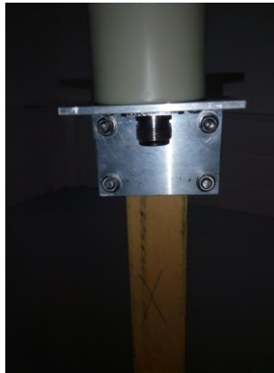
Figure 6-9 : Picture of the fastening system with the 4 gear clamped.
